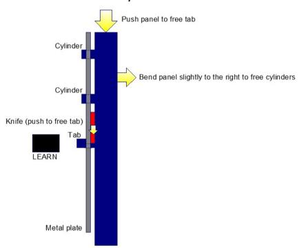
By the way, removal of the 'corrugated' plastic panel (which could be a next step after removal of the two side panels) isn't very easy either, due to its various, rather vulnerable tabs. However, depending on which part of your BCF/BCR you want to fix, it may not be necessary to remove the corrugated panel.
