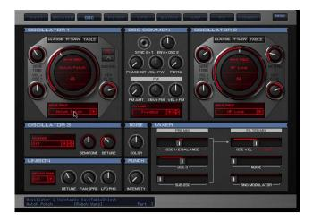
The two big dials represent Oscillators 1 and 2. The graphic in the centre of each represents the current waveform – grab it with the mouse and move it around to 'morph' between
