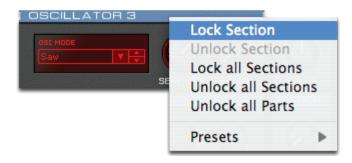
Section locking is a unique and versatile tool to import certain aspects of a patch into another one. It enables Virus Control user to decide which aspect of a given sound is changed when browsing through patches.
