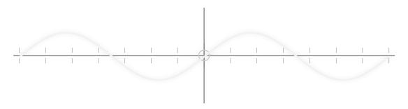
In TIOS 4.5 each of the 3 LFOs can now be selected in unipolar mode. This means that the modulation only occurs in one direction away from the current value of the target parameter.
