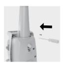
Insert the 2 screws and tighten using a cross head screwdriver.
