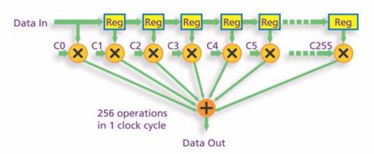
Figure 1: FPGAs Parallel Approach to DSP Enables Higher Computational Throughput
