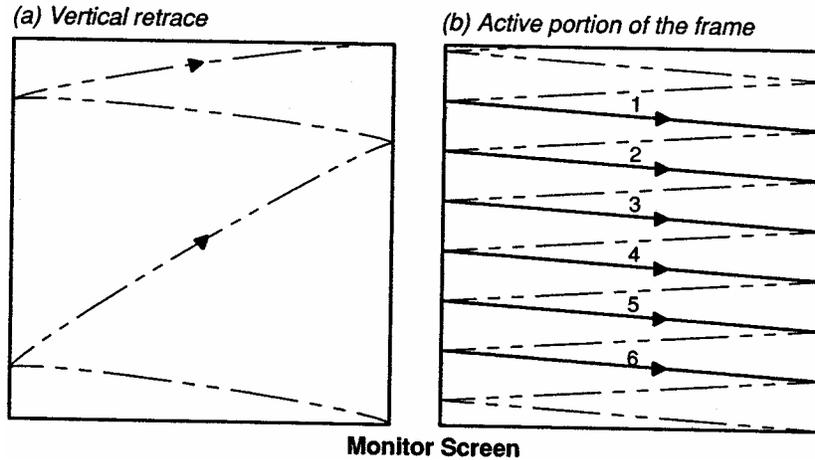
**Figure 2: Non-Interlaced Raster Scanning Pattern**
