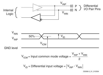
Figure 1: Differential Input Voltages
