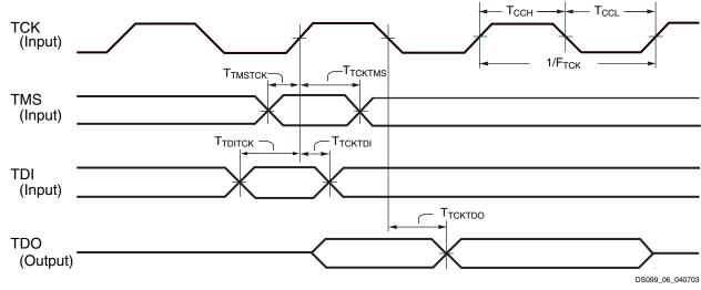
Figure 8: JTAG Waveforms
