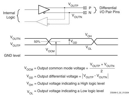
Figure 2: Differential Output Voltages
