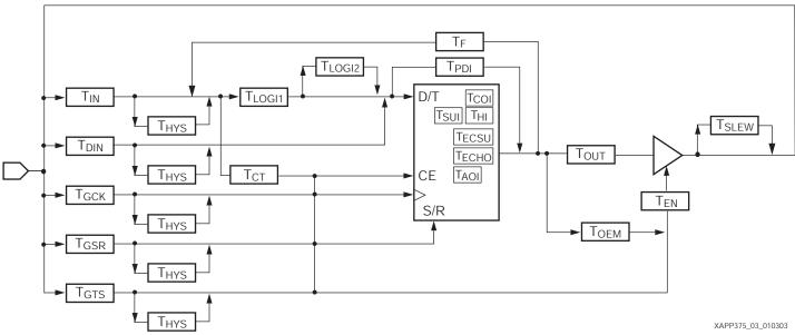
Figure 11: CoolRunner-II CPLD Timing Model
