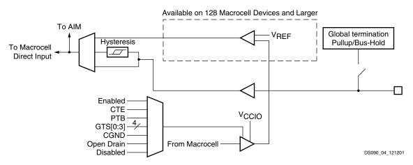
Figure 4: CoolRunner-II CPLD I/O Block Diagram
