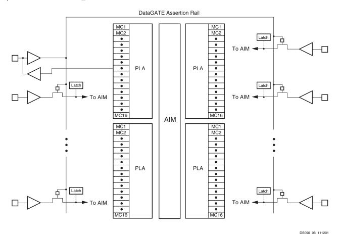
Figure 6: DataGATE Architecture (output drivers not shown)
