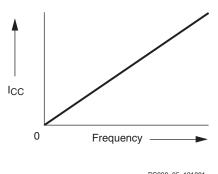
Figure 5: CMOS I<sub>CC</sub> vs. Switching Frequency Curve
