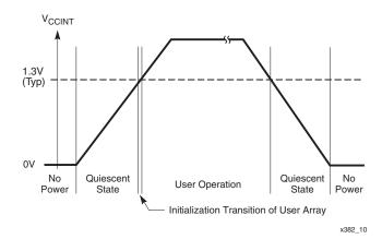
Figure 12: Device Behavior During Power Up
