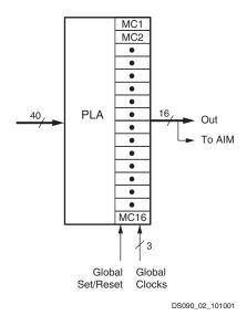
Figure 2: CoolRunner-II CPLD Function Block
