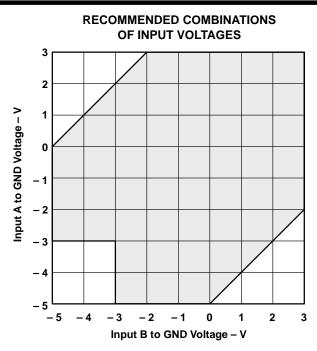
Figure 1. Recommended Combinations of Input Voltages
