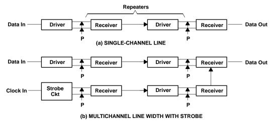
Figure 19. Receiver-Driver Repeaters
