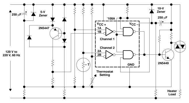
Figure 22. Zero-Voltage Switching Temperature Controller
