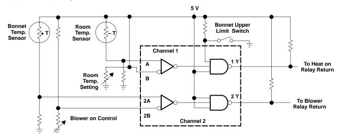
Figure 18. Furnace Control Using SN75108A
