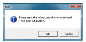
Downloading is performed to open the "Download" window. When downloading is completed normally, the following dialog window opens.
