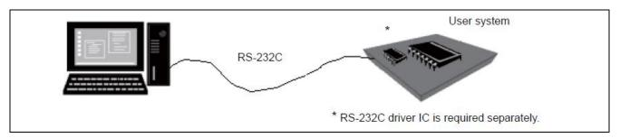
Using RS-232C cable connected to the personal computer (Windows PC), flash memory data in the microcontroller mounted in the user system can be reprogrammed. Note that the user system must have an RS-232C driver for communication with the microcontroller UART.
