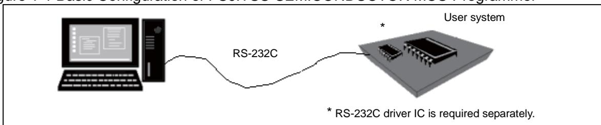
Table 1-1 System Configuration of FUJITSU SEMICONDUCTOR MCU Programmer
