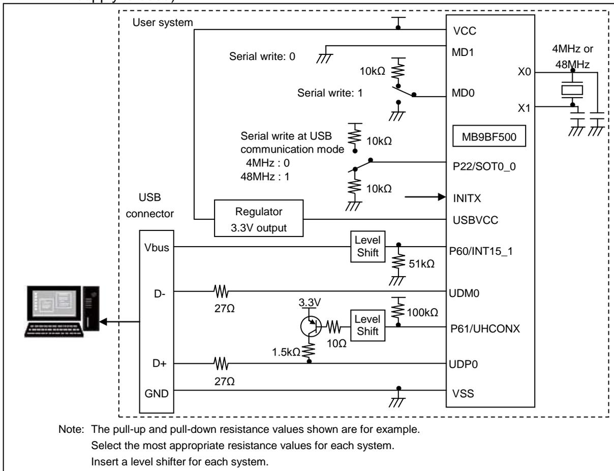
Figure 1-5 Connection example using FUJITSU USB DIRECT Programmer (bus power supply is used)
