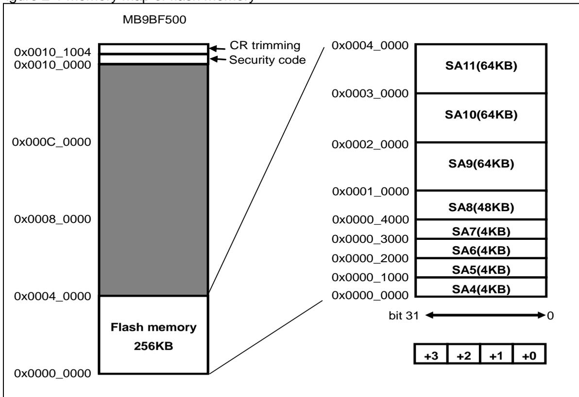
Figure 2-2 Address of security/CR trimming data
