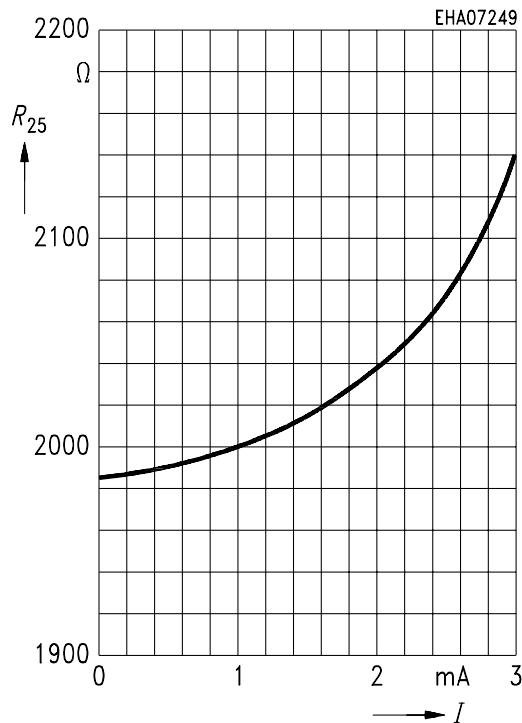
**Sensor Resistance**  $R_T = k_T \times R_{25} = f(T_A)$
