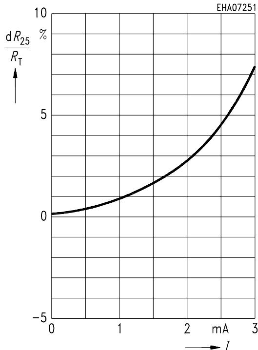
**Typical Deviation of Sensor Resistance from the Basic Resistance  $R_{25}$  ( $I_B = 1\text{mA}$ ) Versus Supply Current**
