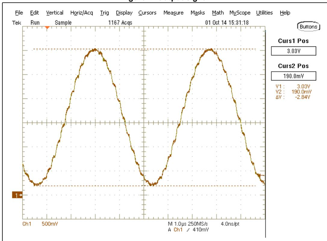
Output swing is not equal to 3.1  $V_{pp}$ , as sampling time is not aligned with the peak of the sine wave signal.
