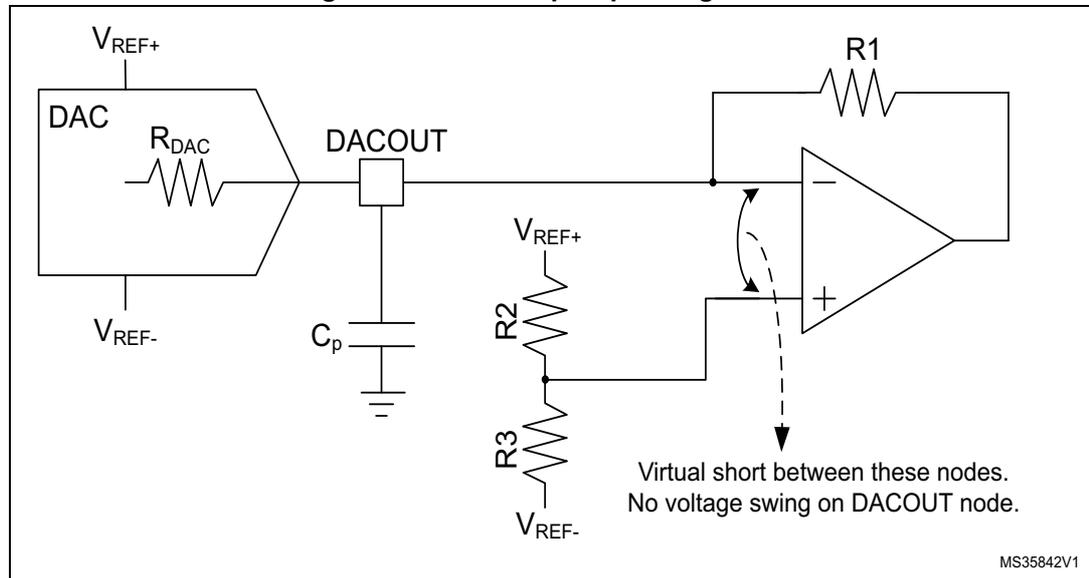
In this configuration there is a minor limitation due to the RC constant, the main limitation being the external OpAmp speed (gain bandwidth and slew rate) and the DAC digital data update rate. There are, however, some disadvantages. The feedback resistor R1 needs to be equal to the  $R_{DAC}$  on chip of the STM32, otherwise it will create a DAC gain error.
