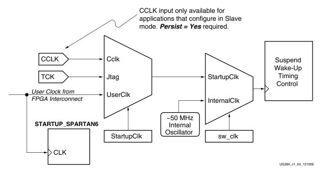
Figure 1-4: Suspend Mode Wake-Up Timing Control Clock Selection
