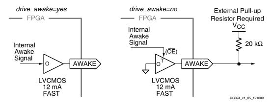
Figure 1-5: AWAKE Output Drive Options if Suspend Mode Enabled
