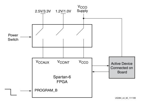
Figure 4-2: Spartan-6 FPGA Power-Off Diagram
