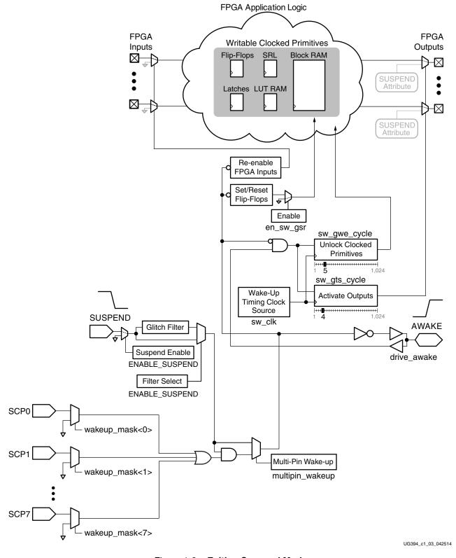
Figure 1-3: Exiting Suspend Mode
