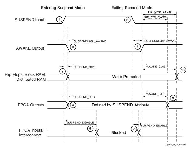
Figure 1-2: Suspend Mode Waveforms (Entering and Exiting)
