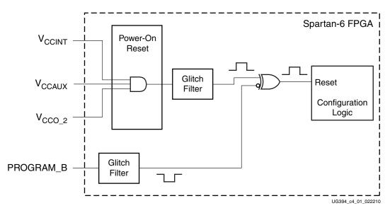
Figure 4-1: Simplified POR Circuit Diagram
