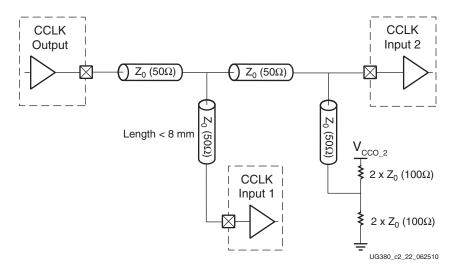
Figure 2-23: Multi-Drop: One CCLK Output, Two CCLK Inputs
