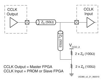
Figure 2-22: Point-to-Point: One CCLK Output, One CCLK Input
