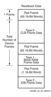
Figure 6-3: Readback Data Stream
