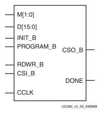
Figure 2-5: Spartan-6 FPGA SelectMAP Configuration Interface
