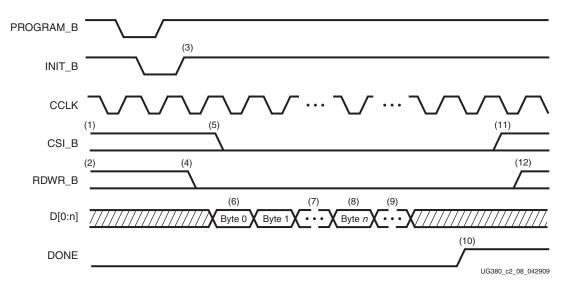
Figure 2-8: Continuous x8 or x16 SelectMAP Data Loading
