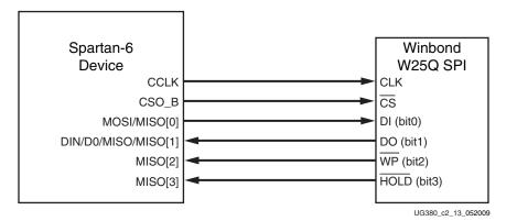
Figure 2-13: Master Serial Quad-Bit SPI Configuration
