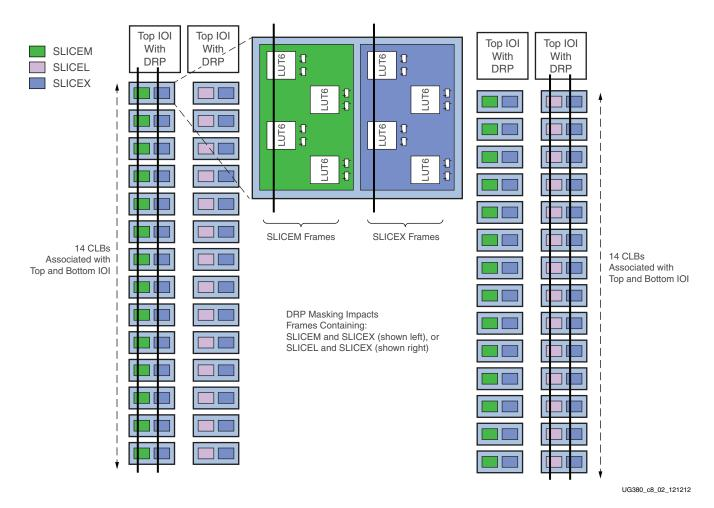
Figure 8-2: CLB Masking with IOI DRP Enabled
