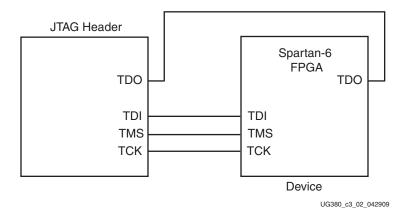
Figure 3-2: Single-Device JTAG Programming Connections
