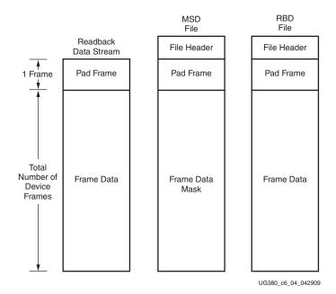
Figure 6-4: Comparing Readback Data Using the MSD and RBD Files
