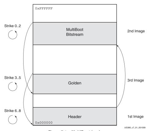
Figure 7-1: MultiBoot Logic
