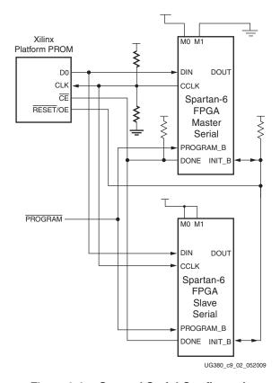
Figure 9-2: Ganged Serial Configuration
