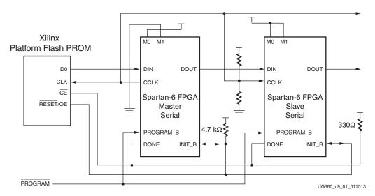
Figure 9-1: Master/Slave Serial Mode Daisy-Chain Configuration
