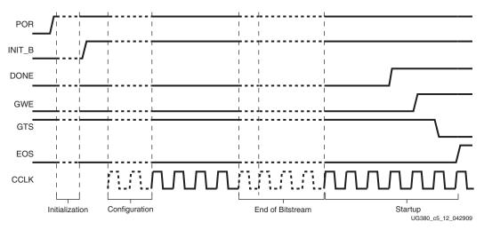
Figure 5-12: Configuration Signal Sequencing (Default Startup Settings)
