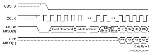
Figure 2-17: Timing Diagram of Winbond SPI Dual-Read Bit Command (3Bh)
