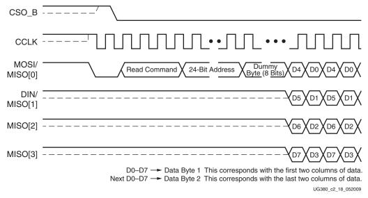
Figure 2-18: Timing Diagram of Winbond SPI Quad-Read Bit Command (6Bh)
