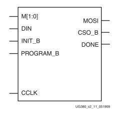
Figure 2-11: Spartan-6 FPGA SPI Configuration Interface
