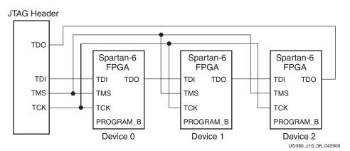
Figure 10-6: Boundary-Scan Chain of Devices
