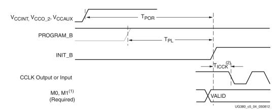
Figure 5-4: Device Power-Up Timing
