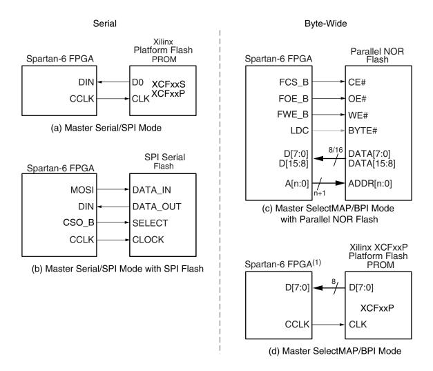
Note: The remaining Spartan-6 FPGAs support XCFxxP Platform Flash PROMs via Master SelectMAP mode. The master serial and the master SPI configuration modes are combined and use the same mode selection. The master SelectMAP and the master BPI configuration modes are combined and use the same mode selection.
