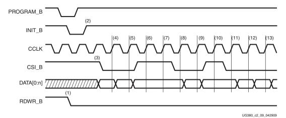
Figure 2-9: Non-Continuous SelectMAP Data Loading with Free-Running CCLK
