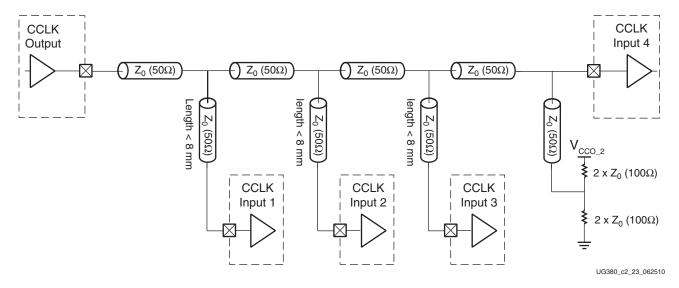
Figure 2-24: Multi-Drop: One CCLK Output, More Than Two CCLK Inputs
