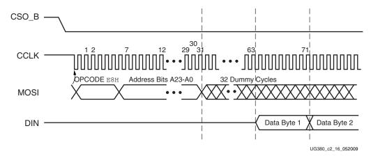
Figure 2-16: Master Serial SPI Timing Diagram (opcode = E8h)
