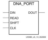
Figure 5-13: Spartan-6 FPGA DNA\_PORT Design Primitive
