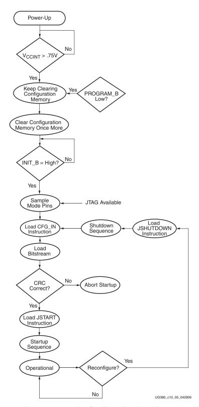
Figure 10-5: Device Configuration Flow Diagram
