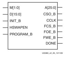
Figure 2-19: Spartan-6 FPGA BPI Configuration Interface
