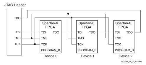
Figure 3-3: Boundary-Scan Chain of Devices
