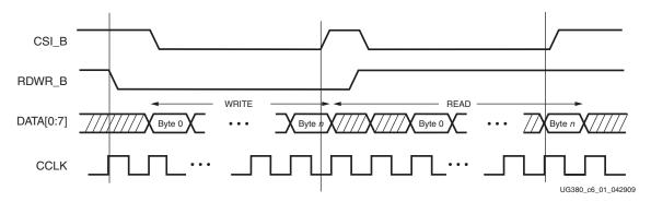
Figure 6-1: Changing the SelectMAP Port from Write to Read Control
