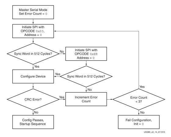
Figure 2-14: Read-Command Looping Mechanism during Initial Configuration
