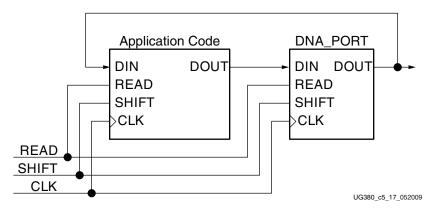
Figure 5-17: Bitstream Specific Code
