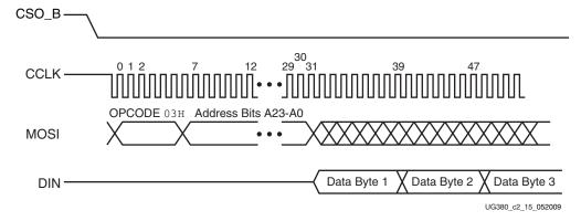
Figure 2-15: Master SPI Timing Diagram (opcode = 03h)
