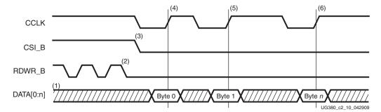
Figure 2-10: Non-Continuous SelectMAP Data Loading with Controlled CCLK
