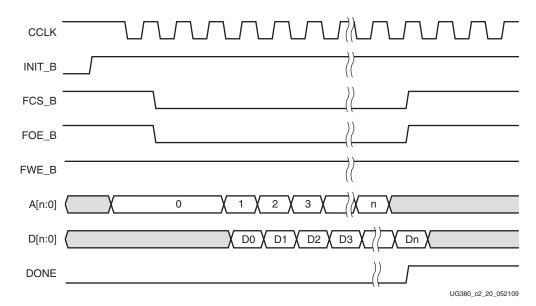
Figure 2-21 shows the BPI configuration waveforms.
