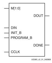
Figure 2-1: Spartan-6 FPGA Serial Configuration Interface
