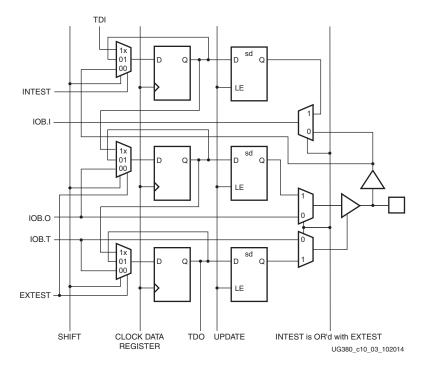
Figure 10-3: Spartan-6 FPGA Boundary-Scan Logic
