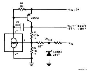
\*Select R3 = V<sub>REF</sub>/583µA. V<sub>REF</sub> may be any stable positive voltage  $\geq$  2V Trim R3 to calibrate
