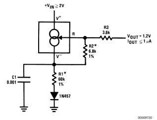
\*Select ratio of R1 to R2 to obtain zero temperature drift
