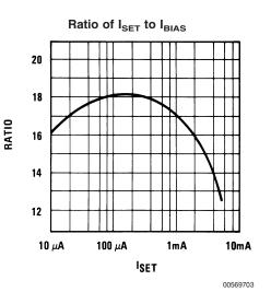
$$I_{\text{SET}} = \left(\frac{V_{\text{R}}}{R_{\text{SET}}}\right) \left(\frac{n}{n-1}\right)$$
