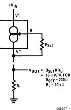
Low Output Impedance Thermometer
