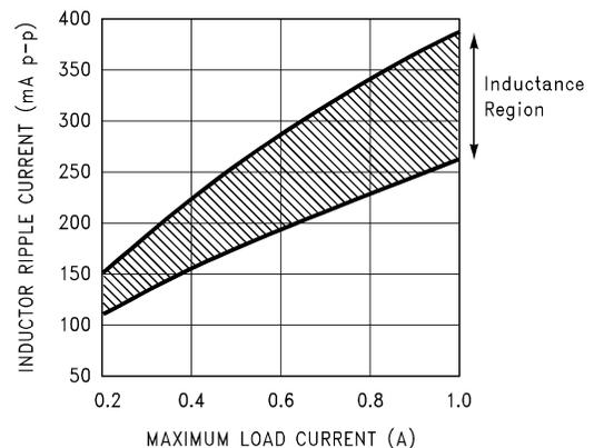
FIGURE 21. Peak-to-Peak Inductor Ripple Current vs Load Current
