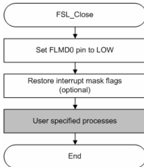
Figure 6-2 Flow of Self Programming End Function
