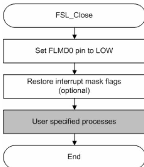
Figure 5-2 Flow of Self Programming End Function
