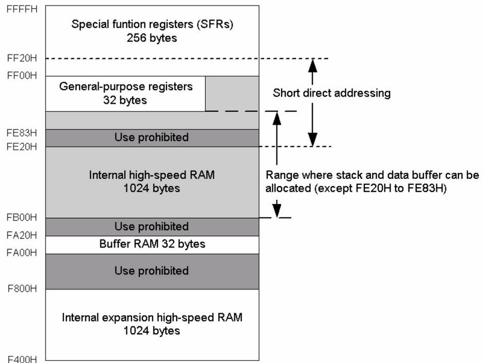
**Figure 2-3 Allocatable Range for Stack Pointer and Data Buffer**
