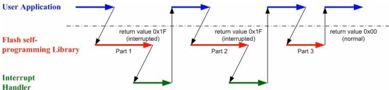
Figure 3-3 FSL Function Process with Resuming Mechanism
