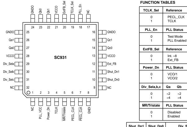
Figure 1. 32-Lead Pinout (Top View)
