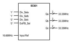
Figure 6. Single Frequency Configuration
