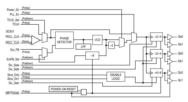
Figure 2. Logic Diagram
