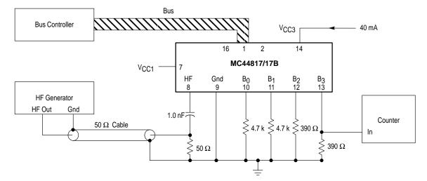
Device is in test mode. B<sub>2</sub>, B<sub>3</sub> are "On" and B<sub>0</sub>, B<sub>1</sub> are "Off". Sensitivity is level of HF generator on 50  $\Omega$  load (without Pin 8 loading).
