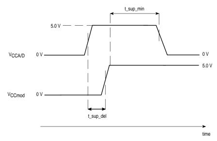
For proper operation of internal reset functions,  $V_{CCA}$  and  $V_{CCD}$  (which must be applied simultaneously) may not be applied after  $V_{CCmod}$ .
