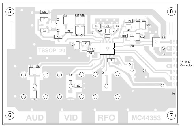
Figure 21. PCB Layout for SO-20L and TSSOP-20 used for Characterization (Bottom Layer)
