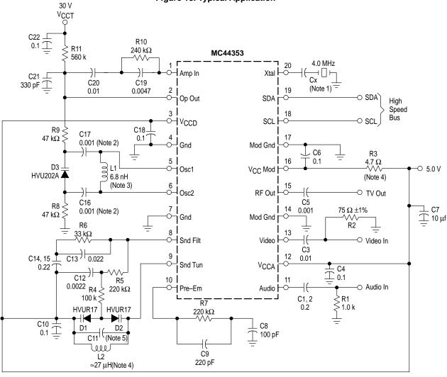
**NOTES:** 1. Cx depends on Crystal Load Capacitance, Crystal resistance < 200  $\Omega$ .
