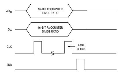
Figure 15. Programming Format for Transmit and Receive Counters (4–Pin Interfacing Scheme)
