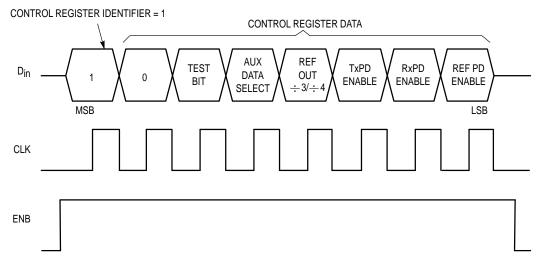
Figure 8. Programming Format of the Control Register
