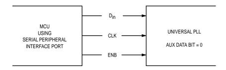
Figure 10. MCU Interface Using SPI
