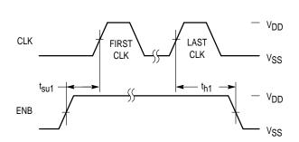
Figure 4. ENB High During Serial Transfer
