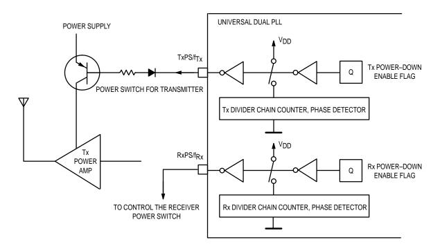
Figure 17. TxPS/f<sub>Tx</sub> and RxPS/f<sub>Rx</sub> Outputs to Control Power Switches of the Transmitter and the Receiver
