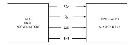
Figure 11. MCU Interface Using Normal I/O Ports with Both D<sub>in</sub> and AD<sub>in</sub> for Faster Programming Time
