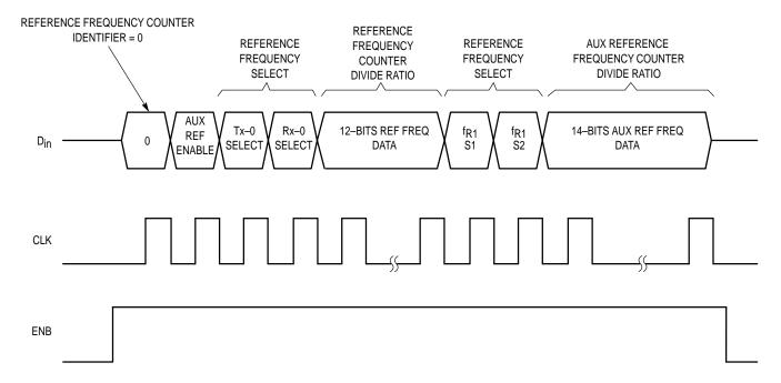
Figure 9. Programming Format of the Auxiliary/Reference Frequency Counters
