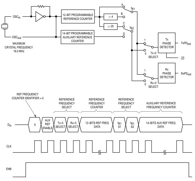
Figure 16. Reference Frequency Counter/Selection Programming Mode
