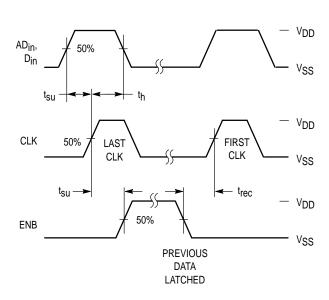
Figure 5. ENB Low During Serial Transfer
