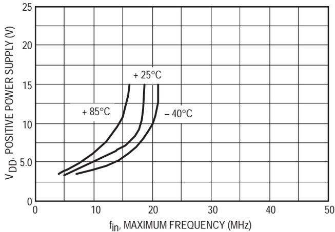
Figure 1. Maximum Divider Input Frequency versus Supply Voltage
