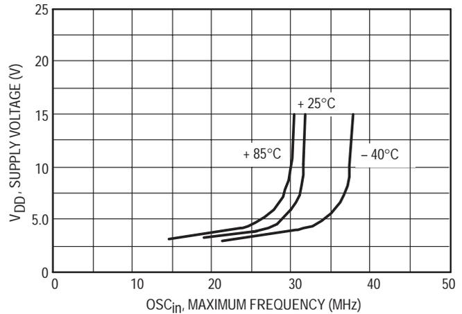
Figure 2. Maximum Oscillator Input Frequency versus Supply Voltage
