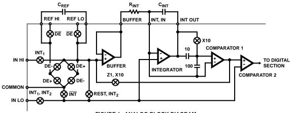
FIGURE 1. ANALOG BLOCK DIAGRAM
