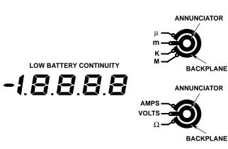
FIGURE 10. MULTIMETER EXAMPLE SHOWING USE OF ANNUNCIATOR DRIVE OUTPUT
