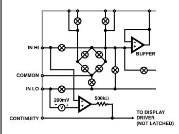
FIGURE 7. "INSTANT CONTINUITY" COMPARATOR AND OUTPUT STRUCTURE
