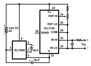
FIGURE 14. POWERING THE ICL7129 FROM A 3.8V TO 6V BATTERY
