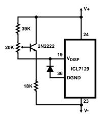
FIGURE 11. TWO METHODS FOR TEMPERATURE COMPENSATING THE LIQUID CRYSTAL DISPLAY
