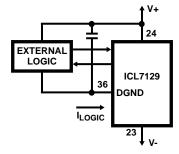
FIGURE 4. DGND SINK CURRENT
