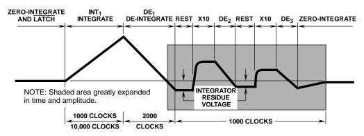
FIGURE 2. INTEGRATOR WAVEFORM FOR NEGATIVE INPUT VOLTAGE SHOWING SUCCESSIVE INTEGRATION PHASES AND RESIDUE VOLTAGE
