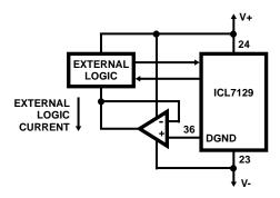
FIGURE 5. BUFFERED DGND
