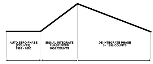
TOTAL CONVERSION TIME = 4000 x  $t_{CLOCK}$  = 16,000 x  $t_{OSC}$
