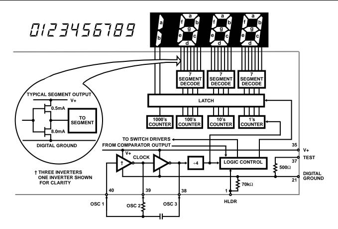
FIGURE 8. ICL7117 DIGITAL SECTION
