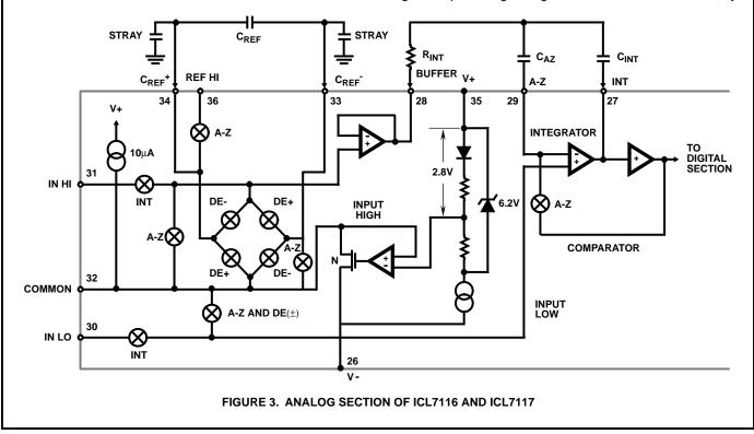
selecting the reference capacitor such that it is large enough in comparison to the stray capacitance, this error can be held to less than 0.5 count worst case. (See Component Value Selection.)
