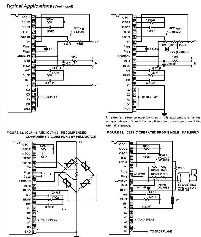
The resistor values within the bridge are determined by the desired sensitivity.
