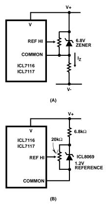
FIGURE 4. USING AN EXTERNAL REFERENCE
