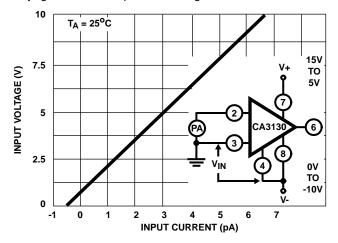
FIGURE 3. INPUT CURRENT vs COMMON-MODE VOLTAGE
