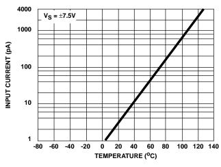
FIGURE 4. INPUT CURRENT vs TEMPERATURE
