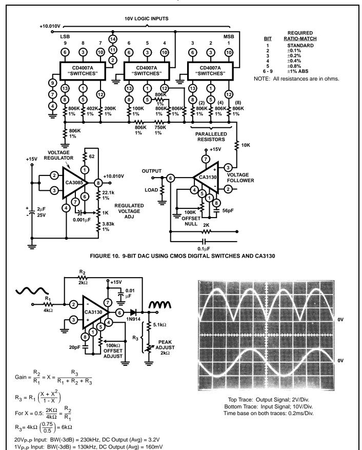
FIGURE 11. SINGLE SUPPLY, ABSOLUTE VALUE, IDEAL FULL-WAVE RECTIFIER WITH ASSOCIATED WAVEFORMS
