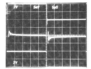
Top Trace: Output Signal; 2V/Div., 5μs/Div. Center Trace: Difference Signa; 5mV/Div., 5μs/Div. Bottom Trace: Input Signal; 2V/Div., 5μs/Div.
