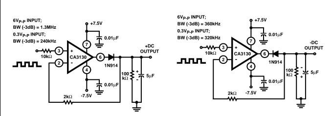
FIGURE 12A. PEAK POSITIVE DETECTOR CIRCUIT FIGURE 12B. PEAK NEGATIVE DETECTOR CIRCUIT FIGURE 12. PEAK-DETECTOR CIRCUITS
