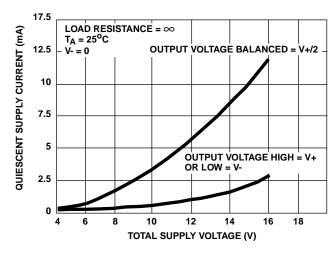
FIGURE 20. QUIESCENT SUPPLY CURRENT vs SUPPLY **VOLTAGE**
