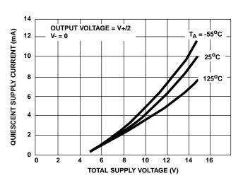
FIGURE 21. QUIESCENT SUPPLY CURRENT vs SUPPLY **VOLTAGE**
