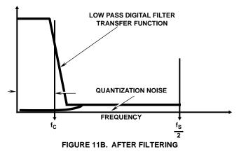
FIGURE 11. IN-BAND QUANTIZATION NOISE BEFORE AND AFTER DIGITAL FILTERING
