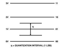
FIGURE 3. CODE EXAMPLE OF A 2-BIT A/D CONVERTER
