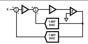
FIGURE 5. SECOND ORDER SIGMA DELTA MODULATOR
