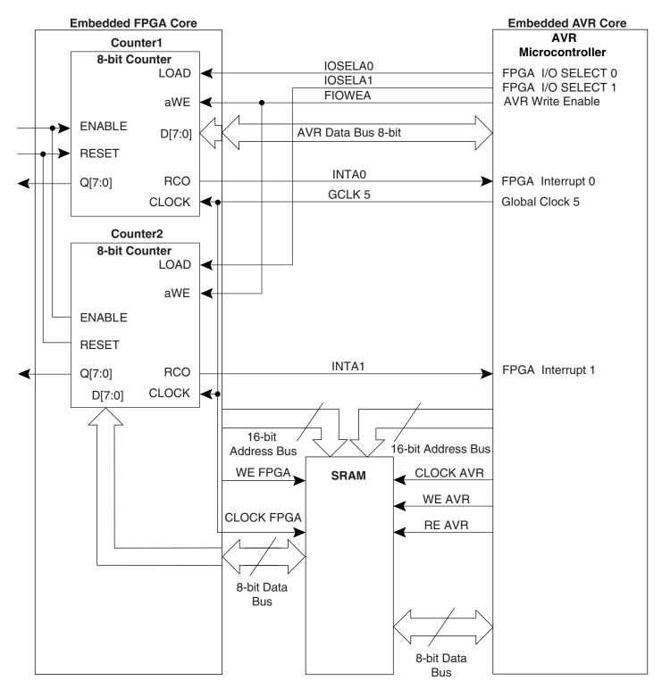
The block diagram shows the connections used in this example, all interface connections are implemented using dedicated resources. This example makes use of the AVR-FPGA Data Bus, two FPGA Interrupts, two I/O Select signals and two SRAM locations.
