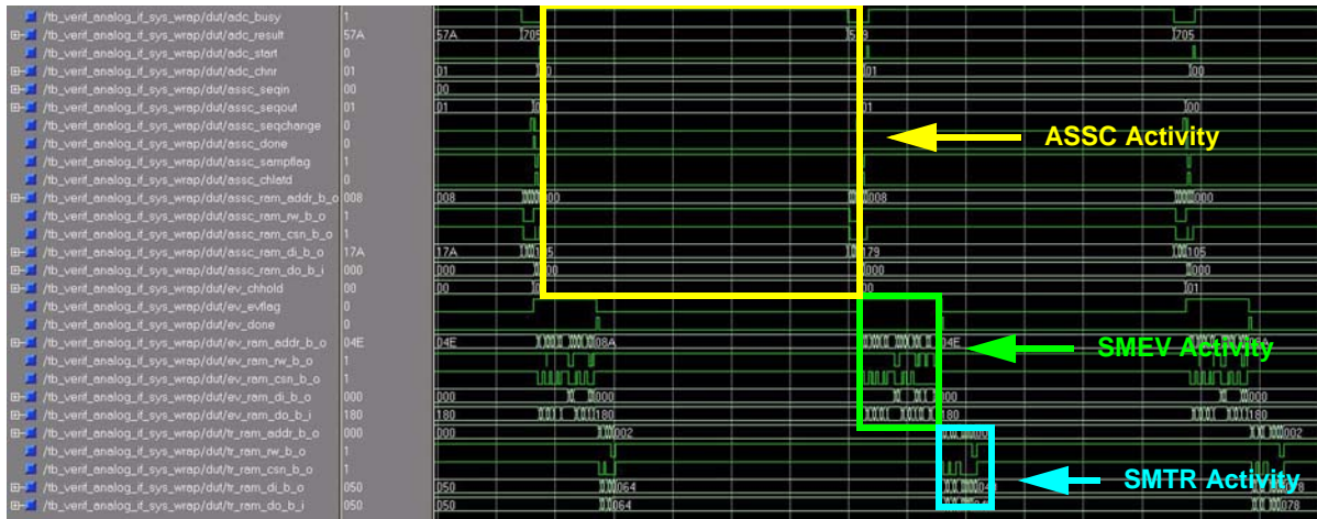
Figure 11-7 • Simulation Result Illustrating Soft IP Events
