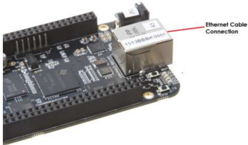
Figure 12. Ethernet Cable Connection
