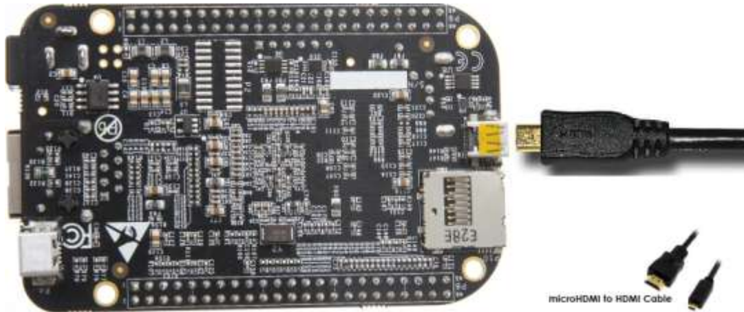
Figure 14. Connect microHDMI Cable to the Board
